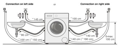
i If the hose holders are used, the possible hose lengths are reduced!
