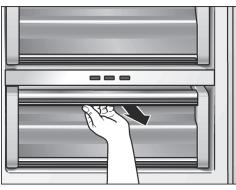
Lift off the filter cover and take out the filter.
