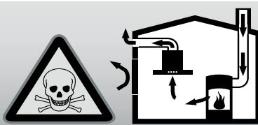
Room air-dependent heat-producing appliances (e.g. gas, oil, wood or coal-operated heaters, continuous flow heaters or water heaters) obtain combustion air from the room in which they are installed and discharge the exhaust gases into the open air through an exhaust gas system (e.g. a chimney).
