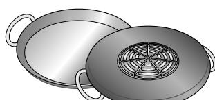
Pans with aluminium areas inserted in the base reduce the ferromagnetic area, so less heat may be supplied and the pan may be difficult to detect or not be detected at all.
