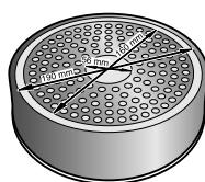
For good cooking results, the diameter of the cookware's ferromagnetic area should match the size of the hotplate. If cookware is not detected on a hotplate, try it on the next smaller hotplate down.
