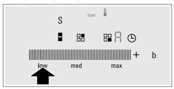
The frying function will have been activated. The ↓ temperature symbol stays switched on until the frying temperature is reached. A signal then sounds and the temperature symbol turns off.
