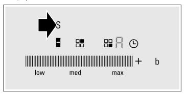
2. Within the next 10 seconds, select the desired temperature setting in the programming zone.
