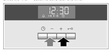
After a few seconds, the oven adopts the settings and switches to standby position. The display shows the time at which the dish will be ready and the  $\blacktriangleright$  arrow is next to the  $\rightarrow$ I symbol. The  $\bigtriangleup$  and  $\odot$  symbols go out. When the oven starts, the cooking time counts down in the display and the  $\blacktriangleright$  arrow is next to the  $\vdash$ I symbol. The  $\rightarrow$ I symbol goes out.
