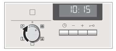
Set the temperature or grill setting using the temperature selector.
