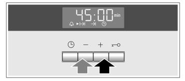
The oven will start up after a few seconds. The cooking time counts down in the display and the  $\triangleright I \rightarrow I$  symbol lights up. The other time symbols go out.
