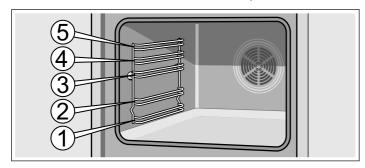
The accessories can be pulled out approximately halfway until they lock in place. This allows dishes to be removed easily.
