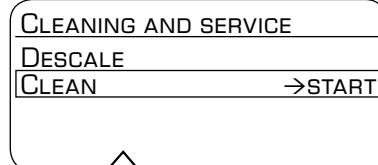
The **start** button **8** flashes while the different cleaning processes are running. The figures on the top right indicate the progress of the programme.
