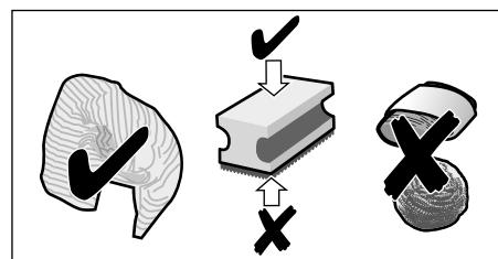
• Always remove any limescale, coffee, milk, cleaning or descaling fluid residue immediately. Such residue can cause corrosion. New sponge cloths may contain salts. Salts can cause rust film on stainless steel and must therefore be washed out thoroughly before use.
