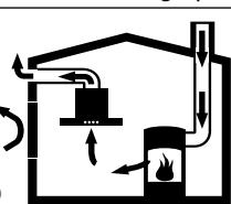
Room air-dependent heat-producing appliances (e.g. gas, oil, wood or coal-operated heaters, continuous flow heaters or water heaters) obtain combustion air from the room in which they are installed and discharge the exhaust gases into the open air through an exhaust gas system (e.g. a chimney).
