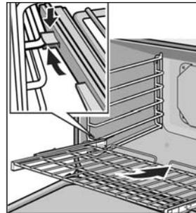
2. Push the rack into the oven, lifting the rack stops over the front of the rack guides.
