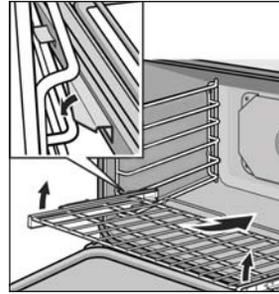
1. Hold the rack on a slight angle. Place the safety hooks under the front of the rack guides.
