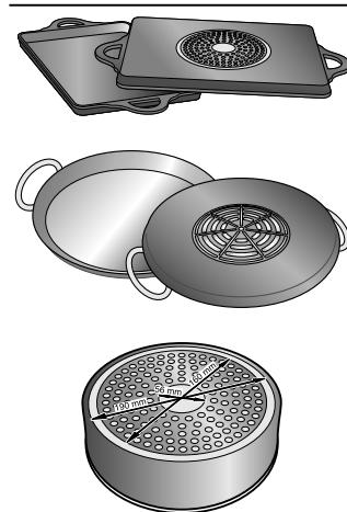
When using large cookware on a smaller ferromagnetic area, only the ferromagnetic zone heats up, so heat might not be uniformly distributed.
