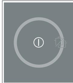
If this symbol appears in the cooking position display, the settings could not be transferred fully. Lift the cookware or move it on the cooking surface. Make the settings for the cooking position again.
