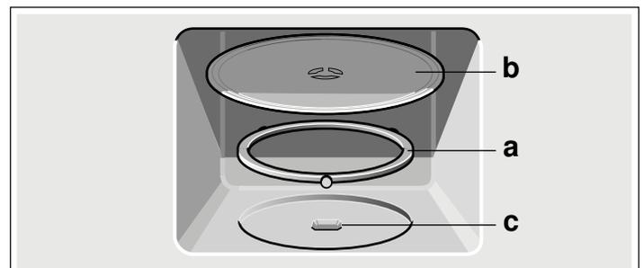
**Note:** Do not use the appliance if the turntable is not in place. Ensure that it is properly slotted into place. The turntable can turn clockwise or anti-clockwise.
