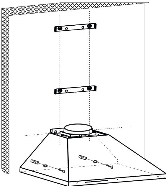
The customer should hang up the hood completely and should at last drill through the hood and the 10mm hole an 8mm hole in the wall. In this 8mm hole he can put a peg and than tighten a screw.
