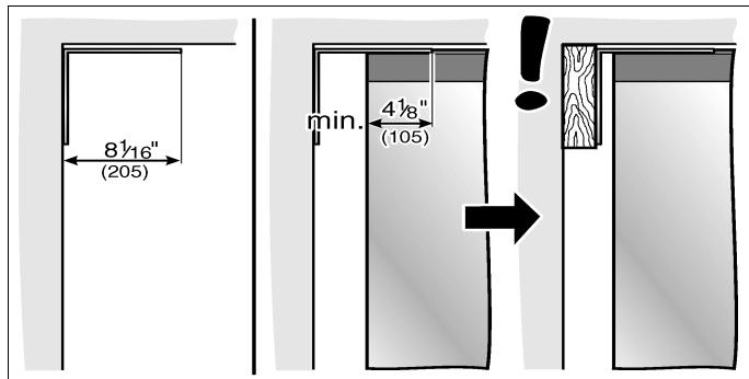
The length of the plank should correspond to the width of the installation niche!
