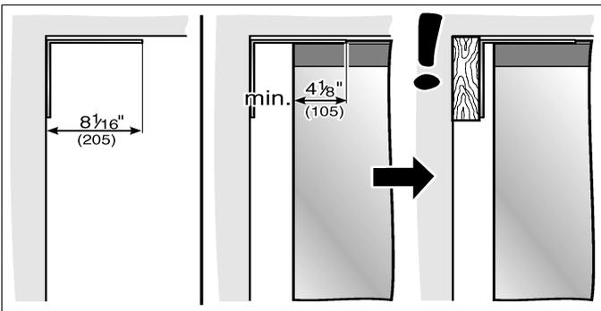
The anti-tip-angles must have a minimum length of  $4\frac{1}{8}$ " (105 mm) over the appliance to ensure a secure stand of the appliance.
