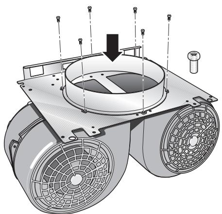
5. Attach the fan on both sides and carefully lift it over the lighting strip.
