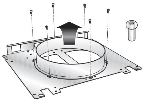
4. Screw the round duct plate to the fan.
