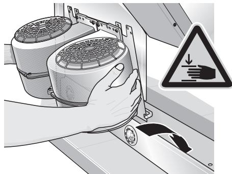
6. Carefully push the fan into the correct position.
