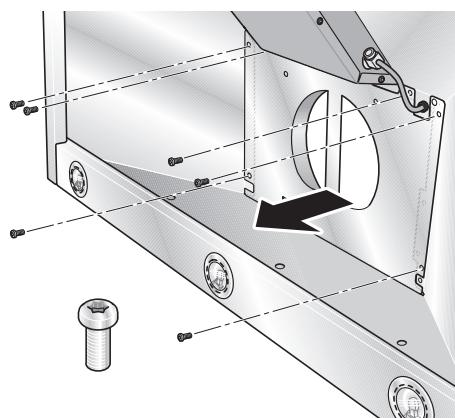
3. Remove the round duct plate.
