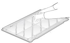
2. Position the filter screen against the housing and push upwards. Push in the lower edge over the lugs and lower the grid into place.
