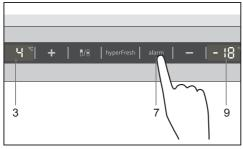
If the temperature inside the freezer exceeds the alarm temperature, "alarm" and the freezer compartment temperature will be indicated on the display and the buzzer (continuous sound) will be actuated.
