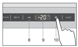
When the setting stops for 5 seconds, the final temperature setting value will be confirmed and stored.
