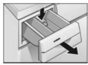
☐ Pull out the detergent dispenser up to the end stop, press down the hollow on the insert and remove the detergent dispenser completely.
