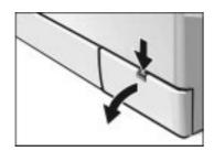
☐ Remove the drain hose from its holder and pull the hose out of the housing.
