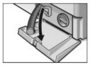
☐ Pull down the closing cap and allow the washing lye to flow into a suitable container.
