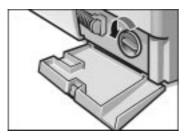
☐ Carefully remove the pump cap.
